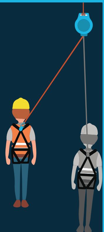
Figure 2 - Illustrates sideways impact with an adjacent vertical structure.
